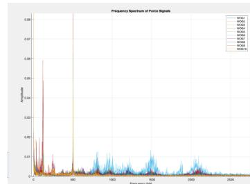
the frequency domain, and the dominant frequency components in the data are displayed. Peaks in the spectrum indicate frequencies at which force variations are most pronounced, in which patterns can be determined that can be associated with the cutting dynamics or mechanical failures impending of the file.
